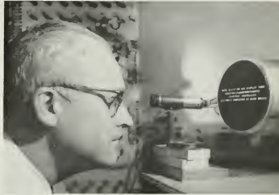
The new RCA electron image tube that converts code to words and figures at high speed is adjusted by Warren H. Bliss at the David Sarnoff Research Center.
