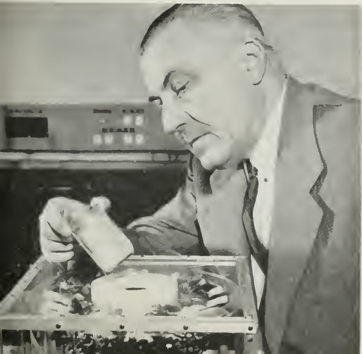
Ice produced in the freezing compartment of the RCA experimental electronic refrigerator is extracted here by Nils E. Lindenblad.
